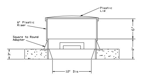
Plastic Riser Can Be Stacked To Grade In 6" Increments
